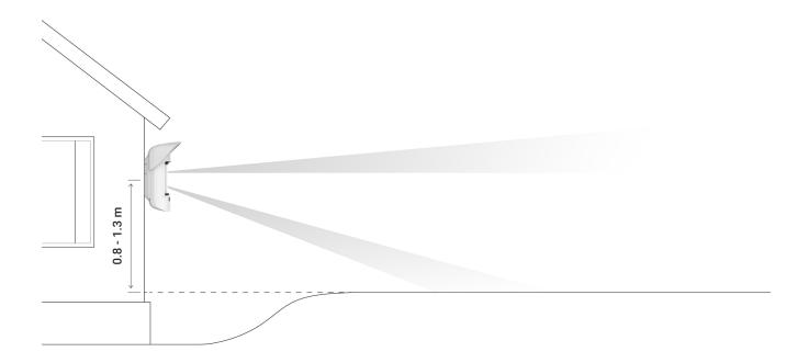
The detector should be installed on a flat, stable surface — for example, on the wall of a house or a solid fence. If the detector is installed on a shaky (unstable) surface, this will result in false alarms.
