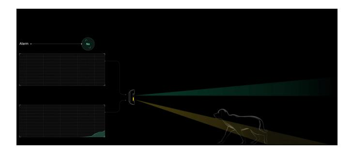
When motion is detected, the LISA algorithm analyses and compares the waveforms of two signals from the infrared sensors in real time. If waveforms are similar, the detector raises the alarm.
